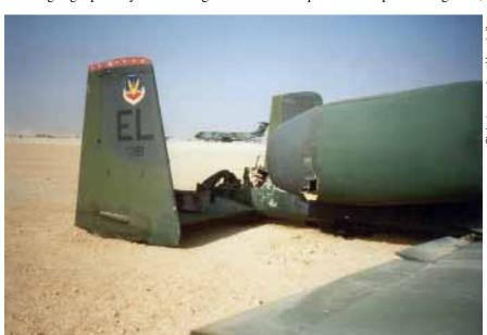
An A-10 shows heavy damage caused by an Iraqi surface-to-air missile during Desert Storm.
